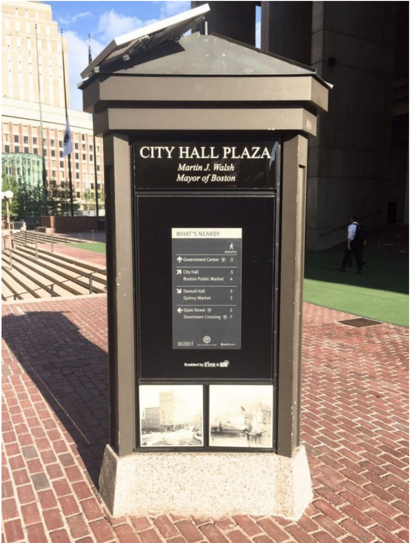
Electronic ink is visible even in bright sunlight, and the e-paper sign is water resistant, making it
